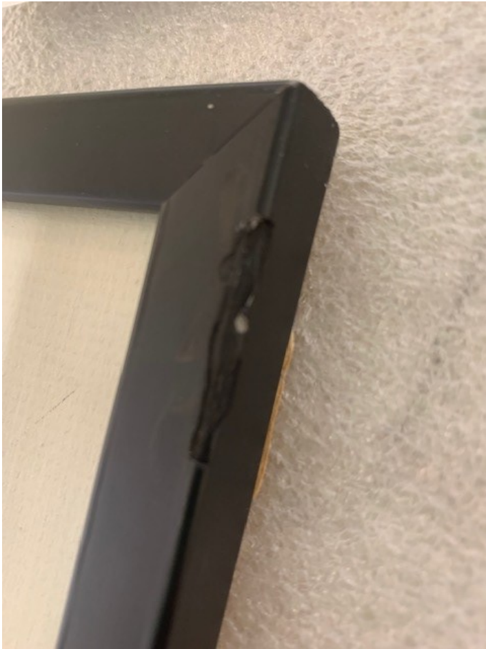
All four images show examples of chipping and scratching along frame.
