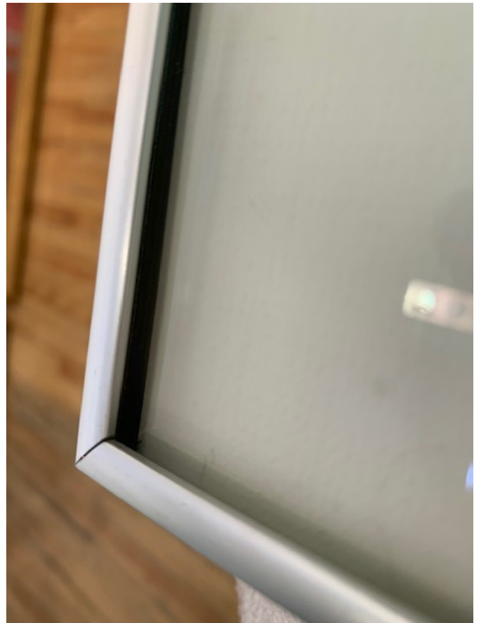
... resulting in gaps between glass and the frame near the corners (only visible when laying flat on a table - NOT when hanging).
